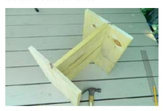
4. Add wood glue to the top of the base and then center the 18" board on top of the base and nail in place with the remaining finishing nails.
